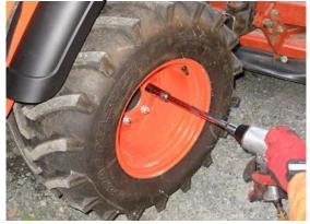
F.You will need a regular socket to mount the wheel spacers on the axle, the heavy wall driver sockets won't fit.
